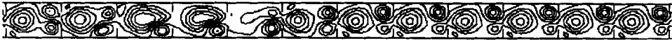
FIGURE 22. A plot of instantaneous streamlines in the (x, y) -plane for a fully developed, asymmetric sinusoidal flow at the point of flow reversal ( t = \text{an integer} ). A two-dimensional numerical simulation was used to obtain the streamfunction distribution, with the spatial periodicity relaxed to twelve cells, as depicted. The flow was started from rest with a small perturbation to allow differences in the flow in each cell to develop. Re and St were 200 and 1.0 respectively. Streamfunction \psi is plotted at intervals of 0.1. The flow is periodic over one oscillation cycle, but it is clear from the figure that the flow is not spatially periodic over each cell of the geometry.
